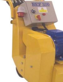
HYD DRIVE SYSTEM WILL ONLY WORK WHEN THE 3PHASE MOTOR RUNS THE CORRECT WAY SO DRUM CUTS THE CORRECT WAY, IF YOU HAVE NO HYD DRIVE CHECK AND CHANGE THE PHASE ROTATION AS ABOVE PICTURE
