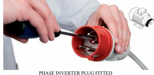
TO BOTH ITEMS TO TURN PHASE ROTATION TO MATCH THE ARROW ON FAN **GUARD SO HYD DRIVE WORKS**
