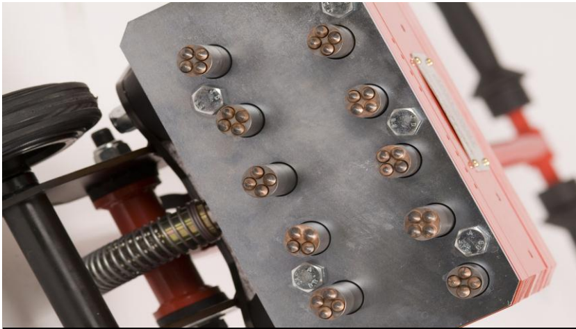
Multi-headed floor scabbler gives 24,000 light blows per minute
