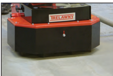
POLISHING CONCRETE FLOORS
