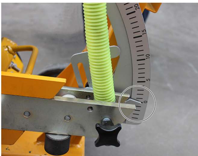
Pointer of the cutting depth display set to 0
