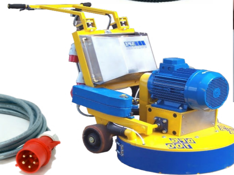
PHASE INVERTER PLUG FITTED TO DFG700 GRINDER TO TURN PHASE ROTATION WHEN USING DIRECTIONAL DIAMONDS SUCH AS PCD
