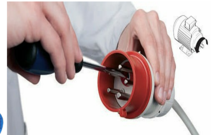
PHASE INVERTER PLUG FITTED TO DFG700 GRINDER TO TURN PHASE ROTATION WHEN USING DIRECTIONAL DIAMONDS SUCH AS PCD
