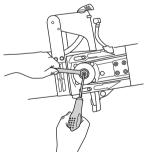
• Remove the cutting arm by pulling it straight out from the machine.
