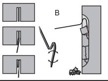
WARNING! When cutting vertically, always cut from the top of the cut and down. Never cut from the bottom of the cut and up. This can cause a kickback and result in personal injury.
